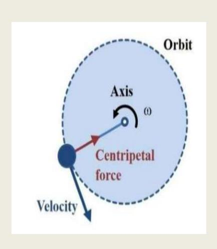
• Centrifugation is a technique of separating substances which involves the application of centrifugal force. The particles are separated from a solution according to their size, shape, density, the viscosity of the medium and rotor speed.
